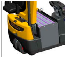
Sideway battery box
